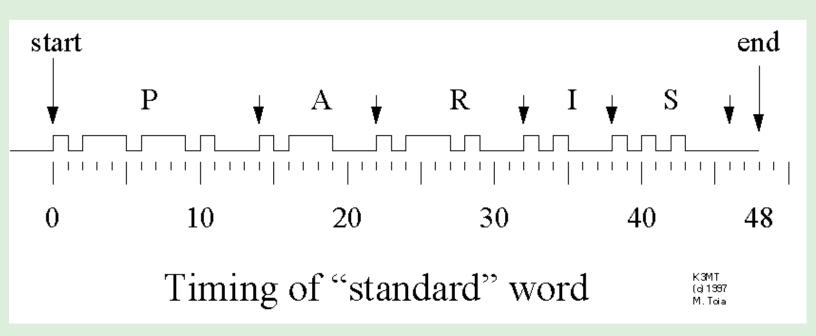
It starts at the "Start" mark. P has the pattern di dah dah dit. Look closely at the graph. Notice the structure of the dits and dahs, and the letter space after the last dit. A small arrow marks the end of P and the start of A. Follow the graph to see the structure of
