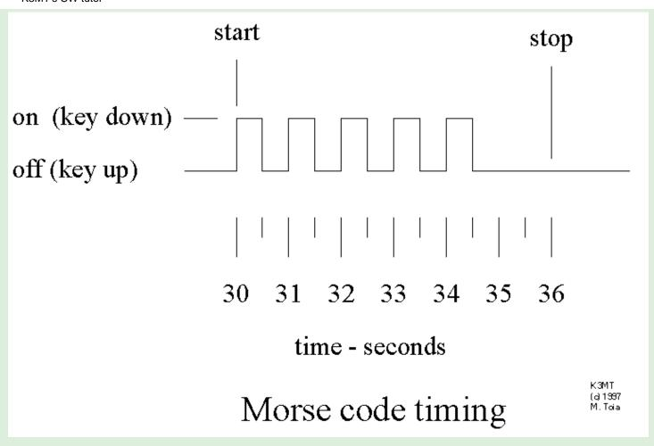
The graph we draw depicts time in seconds passing away along the horizontal axis, from left to right - our time axis always goes from left (the past) to right (the future). The vertical axis shows whether the transmitter is "on" - key "down" - or "off" - key "up".
